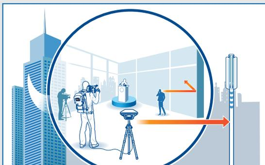
An Xtender was positioned near the window and was connected wirelessly to an LU70. During the test, the combined Xtender / LU70 provided a steady signal of 2Mbps up to 25 meters inside the office enclosed with concrete walls.
