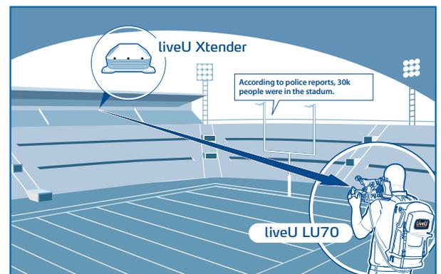
The LiveU Xtender and the LU70 were connected using the wireless connectivity kit to provide aggregated bonded bandwidth. Analysis of internal log files compared the LU70 performance alone versus its performance with a LiveU Xtender with the following results
