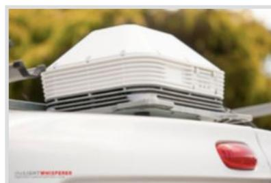
I wanted to just add a footnote about the LiveU Xtender. It is an extra antenna that can support 6 more data SIMs and can be connected by a long cable to the LU500.
